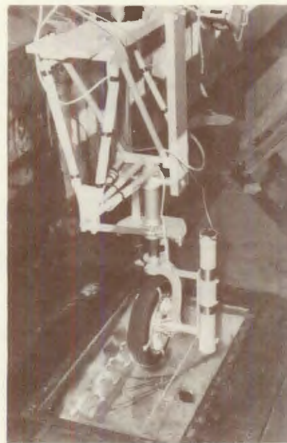
Nosewheel tire on glass track . . . camera beneath
